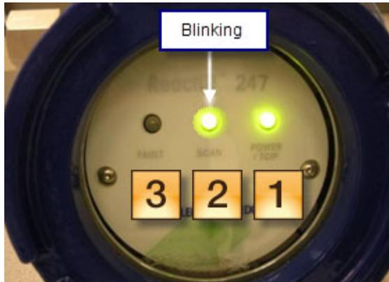
Figure 5-1 ReactIR 247 LED Indicators (fully functional state)
